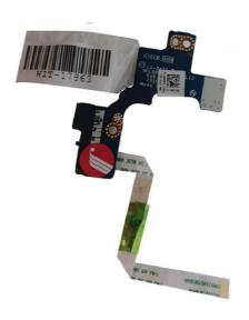
Power Button Circuit Board With Cable For Laptop
