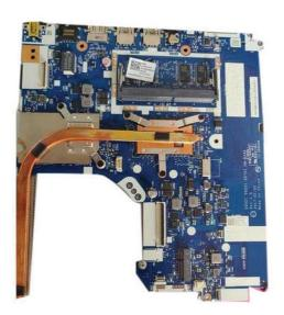
Lenovo Ideapad 320-15ikb Laptop Motherboard With Processor Core i5-7th Gen & Graphics Chip (Refurb)
